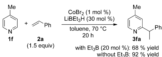
Scheme 4. Reactions of C4-substituted pyridine 1f in the presence and absence of \text{Et}_3\text{B} .
